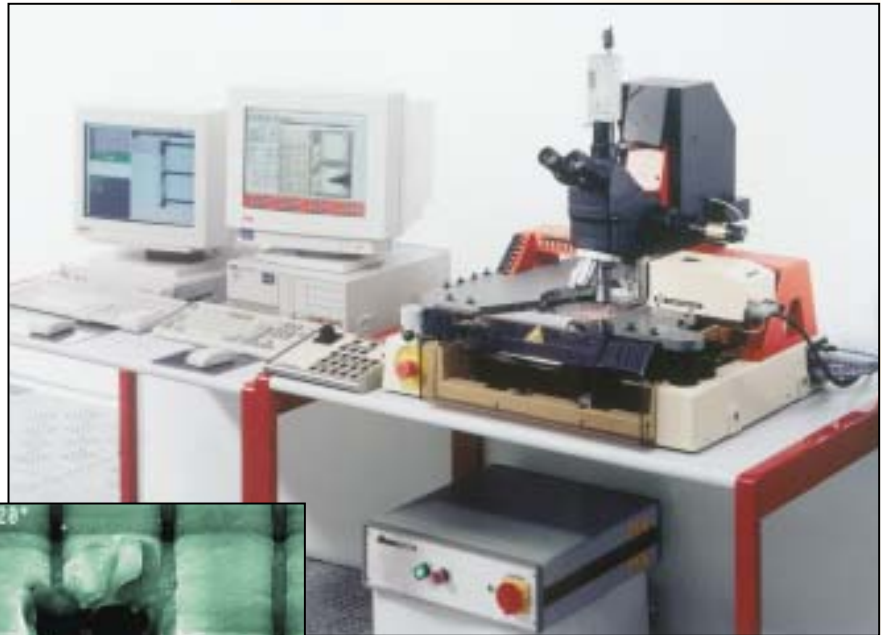
A typical CAD Navigation set-up
