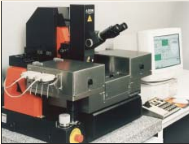
PA200 with ProbeShield® EMC for low signal and low temperature probing
